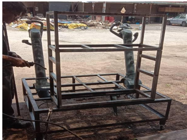
Figure 1: Main structure of the flight simulator
