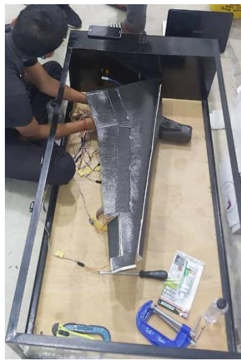
Figure 3: A320 Wing Training Kit with its wiring and being mounted on the metal casing
