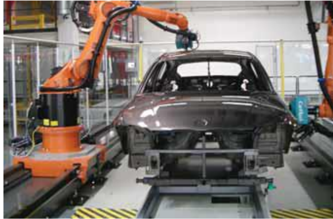
Figure 5: Availability of automated online film thickness measurement using robotic technology
