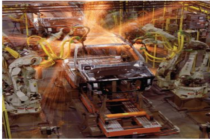
Figure 2: Spot-welding performed by robots on an assembly line [3]
