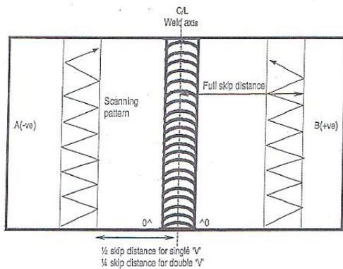
**Figure 3.** Examination Butt Weld with angle beams.
