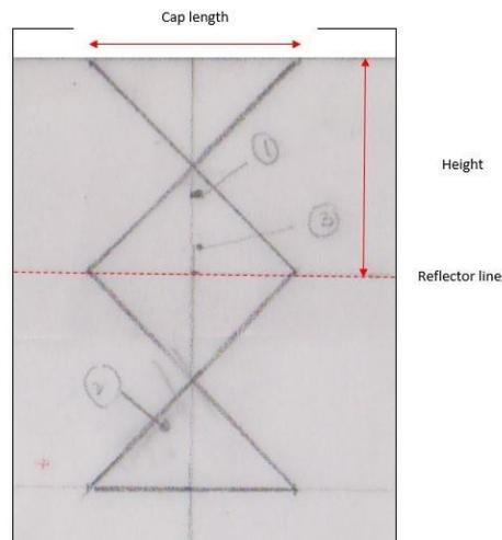
**Figure 10.** Location of defects in Double V.
