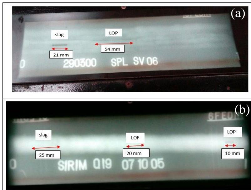
Figure 12. Result of X-ray for (a) Single-V and (b) Double-V
