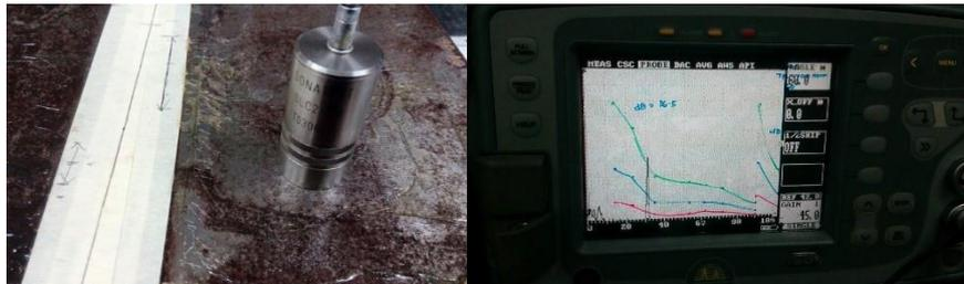
**Figure 1.** Scanning of parent metal with normal probe
