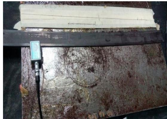
**Figure 4.** Lateral scanning for critical root scanning.
