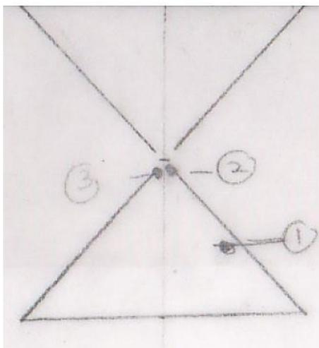
**Figure 9.** Location of defects in Single V.
